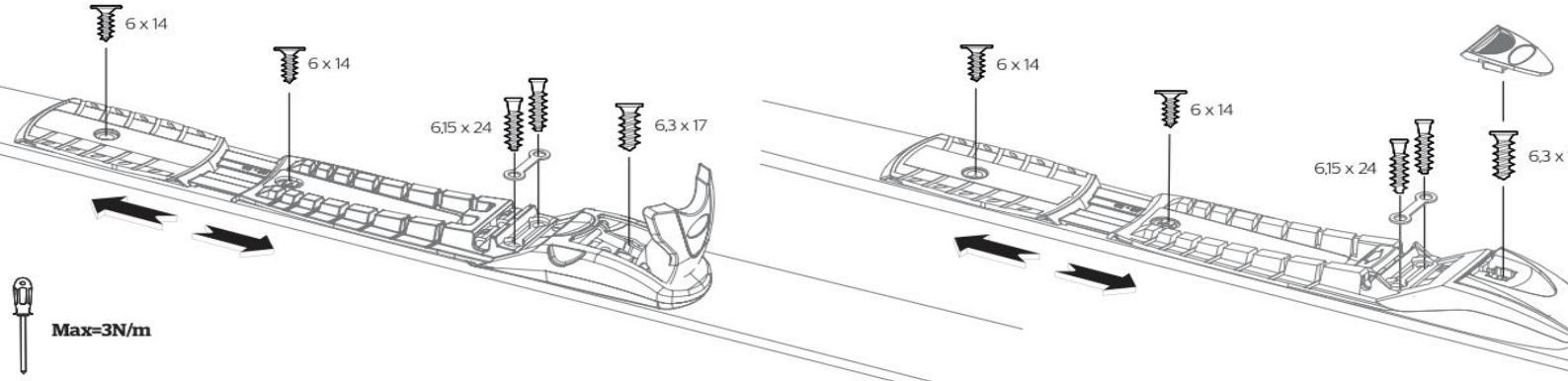
3 Push the flex in place (1) and place stickers to cover up screw holes (2).
